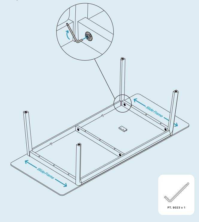
INSTALLING THE METAL BRACKETS.
